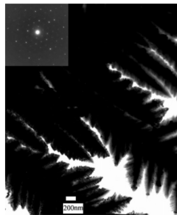
Figure 6. HRTEM and ED of the CuNi dendrite obtained at the potential -1.0 V with an electrolysis time of 2400 s.
